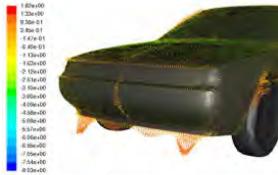
Japan External-aero Competition; New Viscous-hybrid Mesh; 2nd Try sensitivity-to-shape Colored By log10(Shape Sensitivity Magnitude) Feb 24, 2011 ANSYS FLUENT 14.0 (3d, pbrs, ske)
