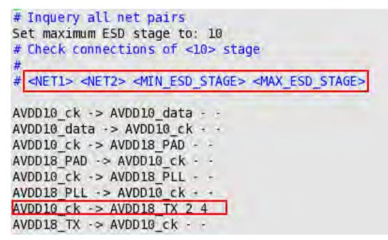
Reports the min/max ESD stage between ESD net pair Minimum 2 stages and up to 4 stages ESD connection between AVDD10\_CK and AVDD18\_TX as shown
