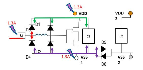
Current Density check rule : 1. Bump2Clamp check: from All pad to corresponding Clamp/Diode zap 1.3A current
