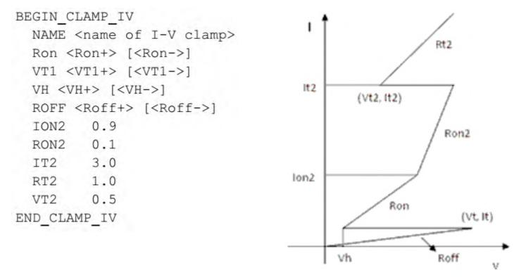
All clamp cells are modeled as resistors with IV curve
