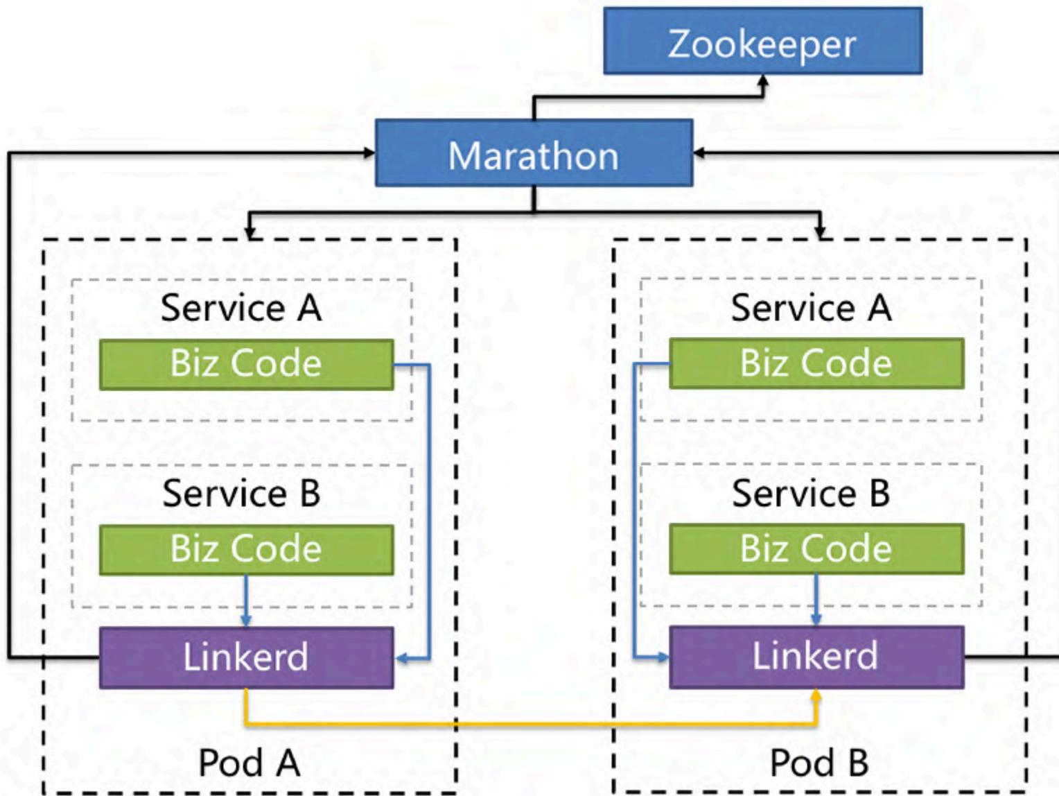
*Linkerd instances form a service mesh, allowing application code to communicate reliably.*
