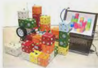
Using physical objects to create a virtual model (Ichida, Itoh, & Kitamura, 2004). As a user adds a physical 'ActiveCube' to the construction, the equivalent virtual model is automatically updated.
