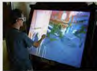
Semi-immersive VR using the Barco Baron workbench (Drettakis, Roussou, Tsingos, Reche & Gallo, 2004).
