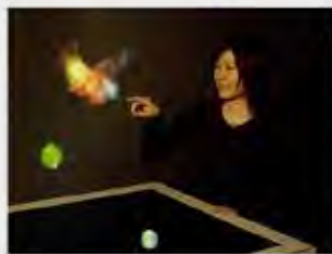
The 'Bubble Cosmos' - 'Emerging Technology' at SIGGRAPH'06. The paths of the smoke-filled bubbles are tracked, and an image is projected into them as they rise.
