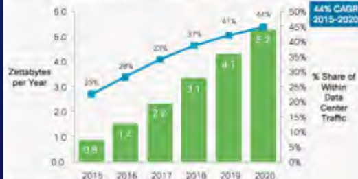
Figure 8. SDN/NFV Traffic Within the Data Center
