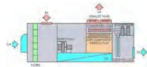
Direct/ Indirect Outdoor Air with Indirect Evaporative Cooling 直接/间接室外空气 加间接蒸发式冷却
