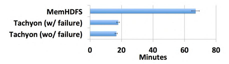
Performance comparison for realistic workflow. The workflow ran 4x faster on Tachyon than on MemHDFS. In case of node failure, applications in Tachyon still finishes 3.8x faster.
